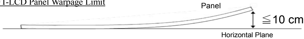
Fig.12 Limit of warpage at handling of panel
