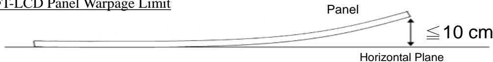
Fig.6 Limit of warpage at handling of panel
